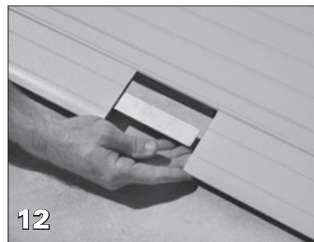
12 Insert the lid hinge splices (M9362) between each section of the lid end support and lid hinge then slide them tightly together.
