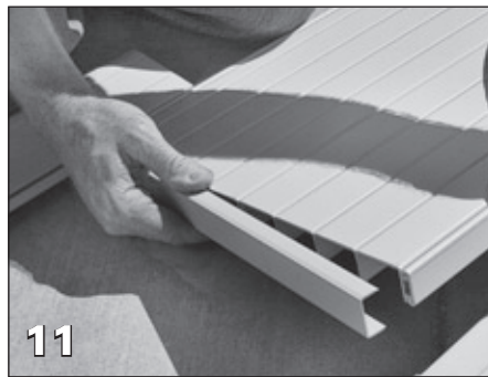
11 Measure and cut motor and non-motor lid ends to fit. Attach the cut cover pieces (M9363) to both sides of the motor and non-motor end lid.
