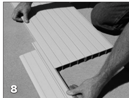
8 Slide the hinge attachment (X0940) and lid hinge onto the lid.
