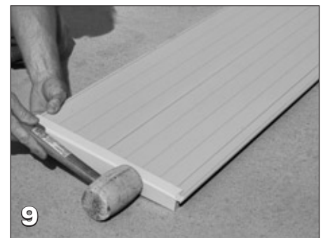
9 Use a rubber mallet to tap on the lid wedges on both sides of the main lid section.
